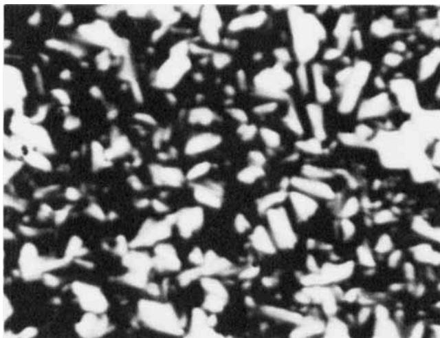
FIGURE 3. Mesomorphic texture of Cu-decylamine complex. See Color Plate VI.
