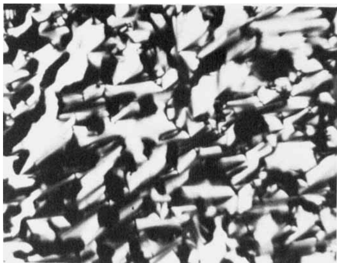
FIGURE 5. Mesomorphic texture of Cu-octadecylamine complex. See Color Plate VIII.
